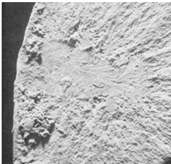
Fig. 11. Polyimide. Scanning electron micrograph (200 \times ) of specimen tested at 80,000 psi.
